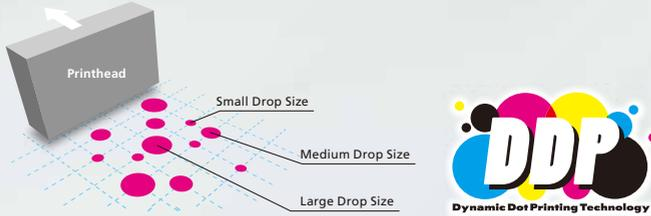
Dynamic Dot Printing Technology controls and optimizes dot size to produce rich, bold and glossy colors with fine details. DDP also creates high density printing without any loss in speed, giving the ColorPainter M-64s backlit film capabilities.
