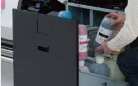
Designed to maximize your print productivity, the ColorPainter M-64s LCIS model comes with a 4.5-liter large-capacity ink reservoir for each color to support continuous high-volume printing. Up to 3 liters of ink can be used continuously without replacing the ink bottles.
